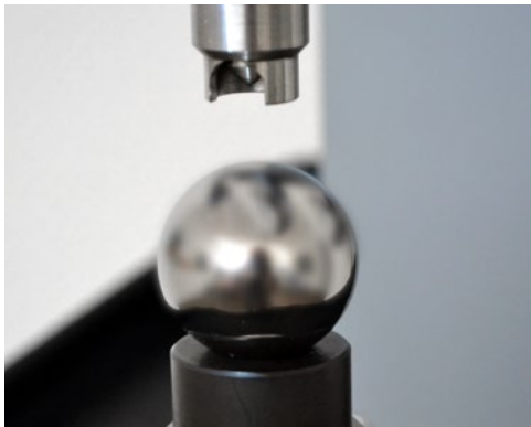
Anvil for ball testing. Therefore the indenter needs to perfectly align with the center of the anvil. Part No - 900001371
