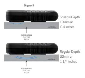
As there is a wide variation in the nominal electrical impedance of different material types, the instrument is provided with three selectable scales which are optimized for testing:
