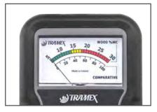
• Lower Scale (0-100) is a comparative scale and may be used for recording and comparing moisture condition in materials other than wood.
