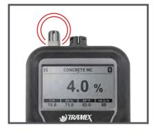
In Equilibrium/Ambient Relative Humidity mode, the Concrete Moisture Encounter X5 determines the capacitance of the RH probe sensor which varies with the relative humidity of the testing environment. The Concrete Moisture Encounter X5 displays this capacitance as a percentage relative humidity. It also measures temperature and displays dew point and humidity ratio.
