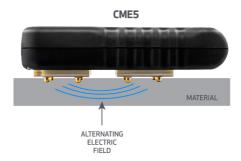
This field penetrates the material under test. A very small alternating current flows through the field. The Concrete Moisture Encounter CME5 detects this current, determines its amplitude and converts it to a moisture content value. By simply pressing the Concrete Moisture Encounter CME5 down on the surface in strategically chosen locations, instant readings can be taken over a large area in the shortest possible time.
