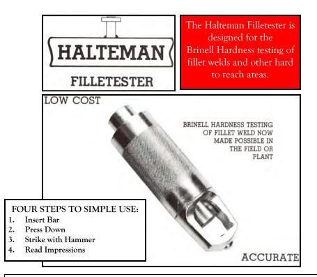
It is used in conjunction with the Telebrineller manufactured by Teleweld, Inc. For easier handling, it is recommended that the standard Telebrineller Test Bars be cut in half. Impressions can be measured by using the 5/8" diameter end of the microscope nose piece.
