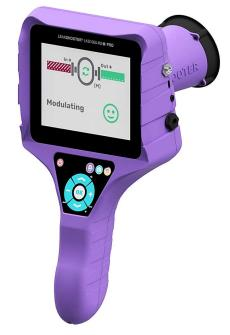
*Example of a modulating "OK" ball float steam trap detected with the STRAPSHOOTER+® program:*
