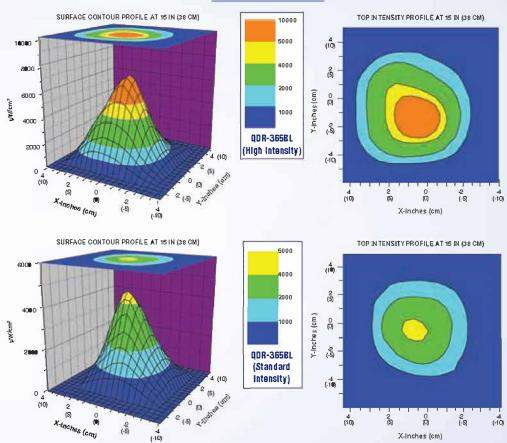
The QDR-365BL is equipped with a faceplate with integral black light filters that reduce the output of wavelengths longer than 400 nm. When in the high intensity mode, the lamp provides a nominal steady-state UV-A intensity of 7,000 µW/cm² at 15 inches (38 cm).
