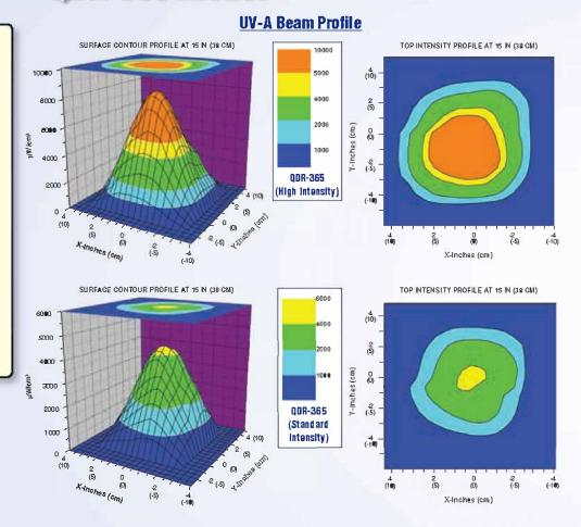
Typical wavelength output profile of QUADRAN™ 365
