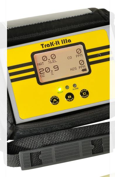
7. The combustible gas scale will automatically range from %LEL to %Volume if so equipped with the 100%v/v (TC) sensor.
