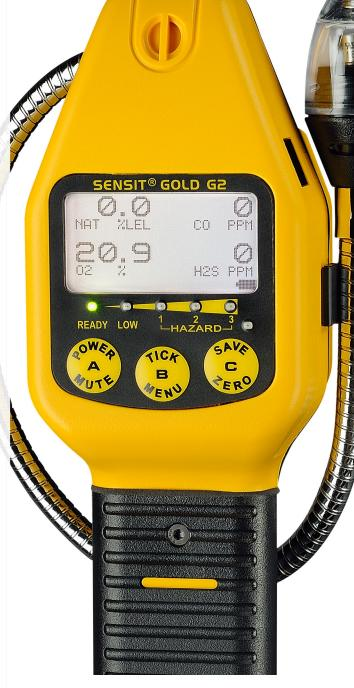
9. Place your finger over the inlet and wait  $\sim$ 5 seconds for "FLOW BLOCKED" to appear on the display. Change cap and "O" rings if it does not show "FLOW BLOCKED".
