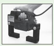
A210 - Heavy Duty A.C. Contour Probe. Strongest A.C. Field Yoke available. Model DA200 available for A.C./D.C. Operation.
