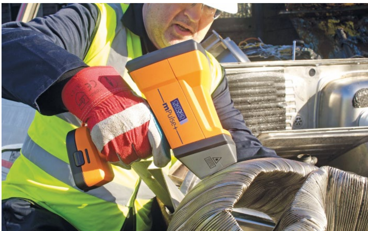
The mPulse+ analyses a wide variety of metal alloys in just one second.
