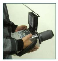
The kit of Ofil's wide field of view lens (wi-FOV) is especially designed to be mounted on DayCor® Rail, DayCor® Ranger, DayCor® Classic and DayCor® Superb and DayCor® ROM inspection systems.
