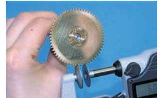
Non rotating spindle type disk micrometers Series 369, 227, 169
