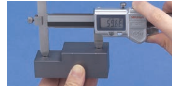
Offset calipers for hole pitch Series 573, 536
