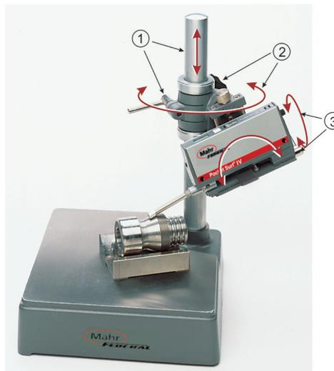
that the bracket with the Pocket Surf unit is tilted, using adjustment ②, to align with the tapered workpiece surface being measured.
