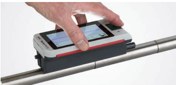
On-site roughness measurement. Measuring in production with the MarSurf PS 10
