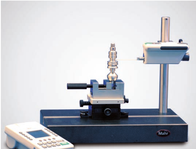
MarSurf measuring station with measuring stand ST-G
