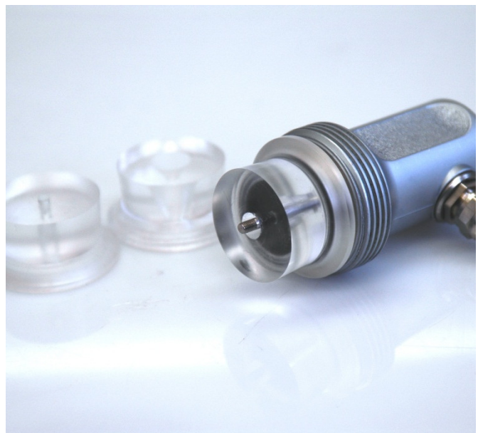
Figure 2: The DYA 5PA32 with modular delay line
