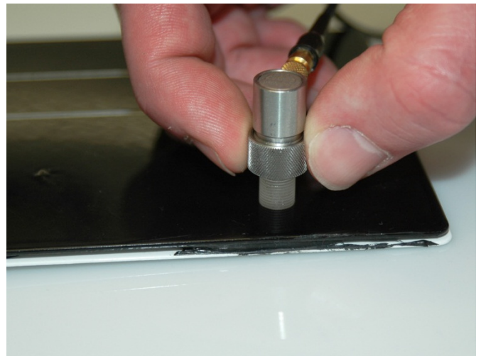
Figure 1: Inspection situation of adhesive bonding
