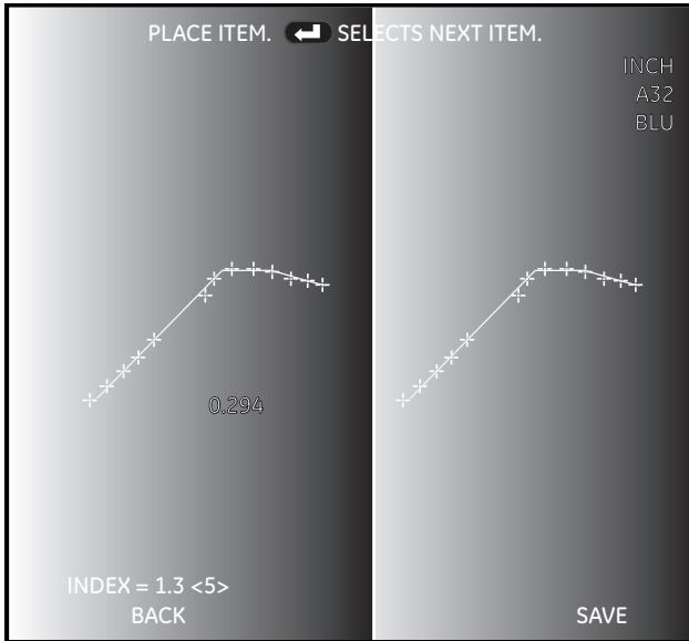
Figure 89: Example of a Depth Measurement
