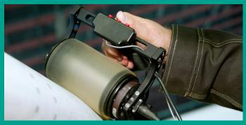
With performance rivaling that of a full immersion C-scan system, our easy-to-use RotoArray gives you faster, more reliable Scan-images, all with the portability of a handheld probe. Together with the Mentor UT, this phased array inspection device allows rapid scanning of a wide variety of materials and components, making ultrasonic inspections even simpler.
