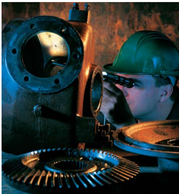
Rigid Borescope inspection of power take-off transmission
