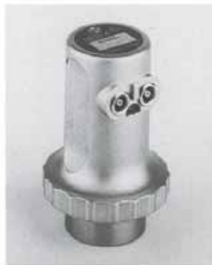
TR probe SEB4 similar to probe DA 0,8G and SEK2C
