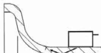
Testing an aluminum wheel rim for cracks with the angle beam probe MSW-QC5 and QC-X45
