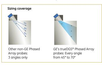
Using the *true*DGS® Phased Array probes can reduce setup times ahead of testing from literally hours to a couple of minutes just by eliminating time consuming reference taking.
