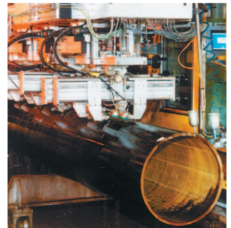
Weld seam inspection on SA-longitudinally welded pipes
