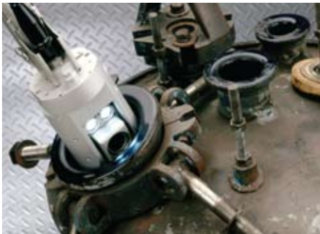
Inspection through a 100mm (3.94 in) \emptyset nozzle
