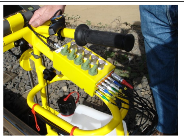
Fig. 4: The distribution box of the SPG 3
