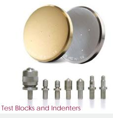
Wilson Instruments offers NVLAP 17025 accredited Rockwell test blocks, diamond indenters, and ball penetrators
