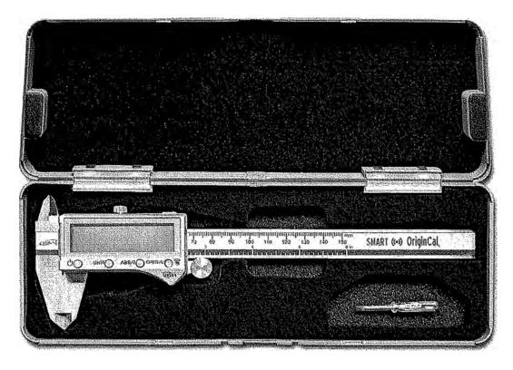
Range 0-6"/150mm, Resolution 0.0005"/0.01mm, Accuracy 0.0001"/0.02mm. Absolute Encoding Technology Memorize Absolute Origin Zero. High Contrast LCD Display and is a **Bluetooth Enabled Device** with **Smart Wireless Data Output**.
