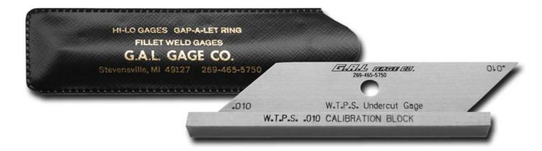
Undercut shall be no more than 0.010 in. (0.25 mm) deep when the weld is transverse to the primary stress in the part that is undercut.
