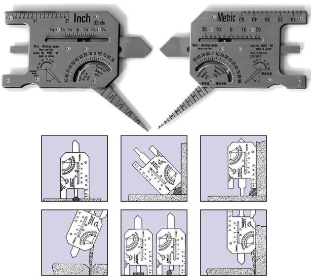
The Combo-Welding Gauge can measure in Inch or Metric all of the following:
