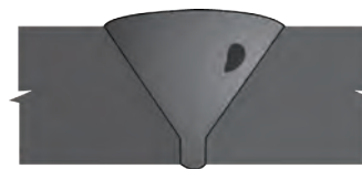
37 Slag Inclusion in Single Vee (weld groove area) UT, RT
