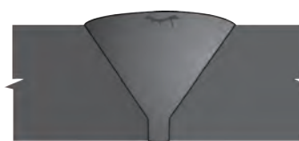
20 Crater Crack (crown stop-start area) MT/PT, UT
