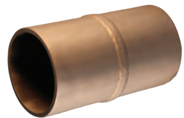
WELDED PIPING 4" SCH160 (0.53" T) x 8" #P109
