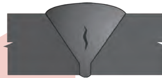
15 Centerline Crack, Single Vee (sub-surface) UT, RT
