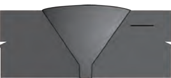
50 Lamination in Single Vee (base metal) UT
