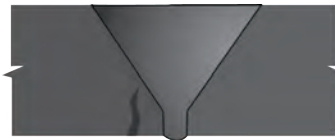
19 Base Metal Crack in Single Vee (bottom HAZ area) MT/PT, UT
