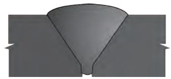
56 Incomplete Root Penetration in Single Vee, VT, UT, RT
