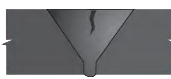
16 Circumferential Crack in Single Vee, flush crown MT/PT, UT
