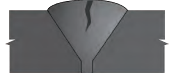
14 Centerline Crack, Single Vee (surface breaking) MT/PT, UT, RT
