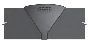
30 Porosity in Single Vee (sub-surface) UT, RT
