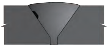
52 Lack of Fusion in Single Vee (crown area) UT
