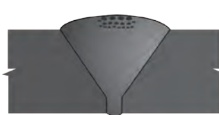
32 Porosity in Single Vee (surface breaking) VT, MT/PT
