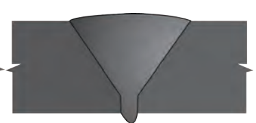
71 Excess Root Penetration in Single Vee VT, RT
