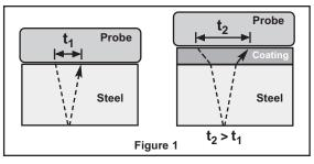
For uncoated materials  $t_1$  relates directly to material thickness. When a material is coated the propagation time is increased and is shown above as  $t_2$ .
