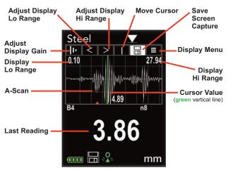
Adjust Display Gain - Adjusts the A-Scan amplitude/sensitivity. Use the (-) and (+) buttons to decrease/increase gain.
