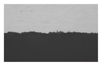
Inside diameter of a steel washer mounted with EpoKwick FC showing no shrinkage gap.
