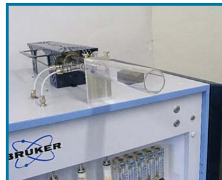
Fig. 2. Quartz tube for heating up the sample material, with a diameter of 30 mm.
