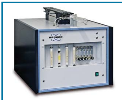
Fig. 1. The "G4 Phoenix DH" analyser for the determination of diffusible hydrogen.
