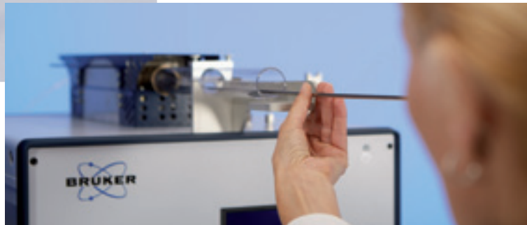
Large diameter (Ø 30 mm) for 1-inch samples like used in AWS A4.3
