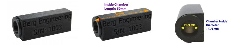
The BE-ZeroG1 Zero Gauss Chamber provides an extremely low and homogenous magnetic field for zeroing your Gaussmeter. The chamber features extremely high magnetic permeability material. This allows for very high levels of attenuation in low intensity magnetic fields.
