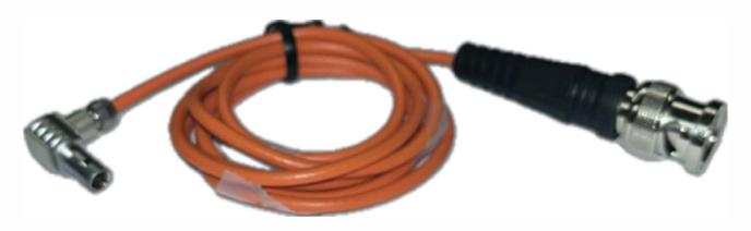
The ORNG-RA114-3 is a short-length ultrasonic cable designed for high-performance signal transfer in flaw detection and thickness measurement applications. This 3-foot cable features a LEMO 00 right angle plug to conserve space in tight setups and a BNC straight plug for easy integration with most ultrasonic testing equipment. Built with RG-174 coaxial cable and a bright orange outer jacket, it delivers low-loss performance and visibility in industrial environments.
