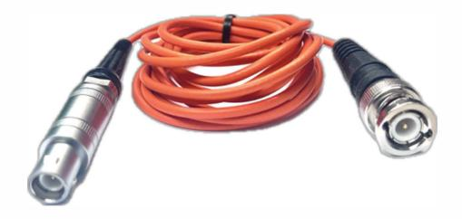
The ORNG-120 is a high-visibility, 6-foot ultrasonic flaw cable constructed with RG-174 coaxial cable. It features a LEMO 01 straight connector on one end and a BNC male plug on the other, offering seamless compatibility between LEMO-equipped probes and BNC-input flaw detectors or instruments. Built for precision NDT applications, it ensures stable 50-ohm signal transmission and is ideal for indoor labs or on-site inspections. Its bright orange jacket improves safety and cable management.
