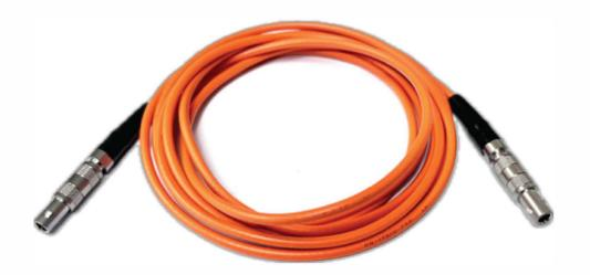
The ORNG-118 is a precision ultrasonic flaw detection cable designed with LEMO 00 straight connectors on both ends and built using RG-174 coaxial cable. Its 6-foot length makes it ideal for benchtop or portable NDT setups. The high-visibility orange jacket improves safety and identification in busy testing environments, while the 50  $\Omega$  impedance ensures accurate and consistent signal transmission critical for ultrasonic flaw detection applications.
