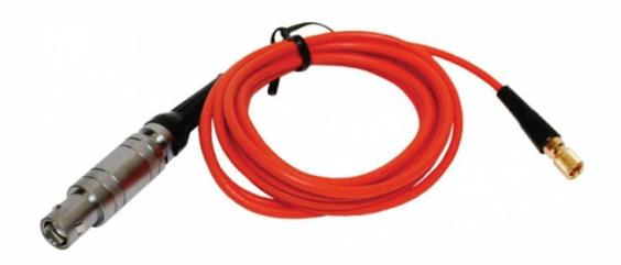
The ORNG-115 ultrasonic flaw cable is a high-performance, 6-foot RG174 coaxial cable configured with a LEMO-1 straight connector and a Microdot straight connector. Designed for precision in ultrasonic non-destructive testing (NDT), this cable supports reliable signal transmission with excellent shielding and durability. Its flexible construction and bright orange jacket make it well-suited for lab, field, and industrial inspection environments.
