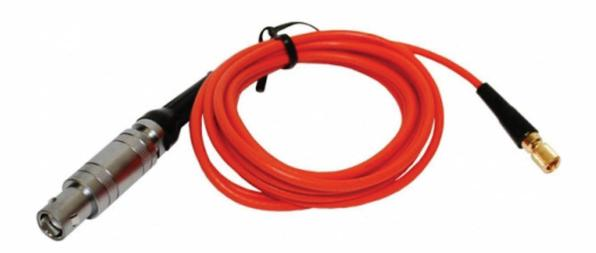
The ORNG-115-3 is a 3-foot, high-performance ultrasonic flaw detection cable built with RG-174 coaxial cable. It features a LEMO-1 straight connector to a Microdot male plug, designed for precision signal transmission in non-destructive testing environments. Its compact length and durable construction make it ideal for portable, bench, and field-based NDT systems.
