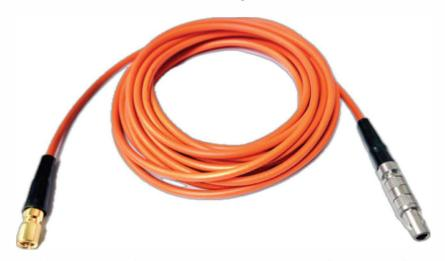
The ORNG-114-12 is a high-quality, 12-foot ultrasonic cable featuring a LEMO 00 straight plug and a Microdot connector, built for precision flaw detection and thickness gauging. It uses RG-174 coaxial cable for flexibility and consistent signal transmission, with a bright orange jacket for visibility in industrial and lab settings. The extended length supports field inspections or setups that require longer reach while maintaining signal integrity.
