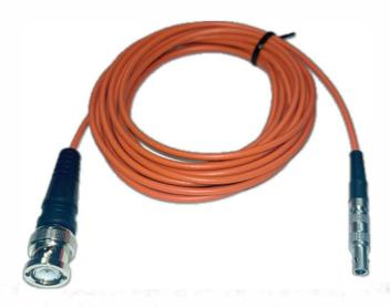
The ORNG-113-12 is a 12-foot ultrasonic flaw detection cable constructed with high-quality RG174 coaxial cable and terminated with a LEMO 00 straight connector on one end and a BNC male connector on the other. The bright orange jacket ensures highly visible cable identification and safety in lab and field environments. This durable cable delivers consistent 50-ohm signal transmission with low loss, making it well-suited for precision ultrasonic testing across a variety of NDT applications.
