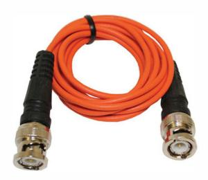
The ORNG-112-4 is a 4-foot ultrasonic flaw detection cable made from RG174 coaxial cable with BNC male plugs on both ends. Its bright orange jacket ensures high visibility and safe handling in both laboratory and field environments. This cable delivers consistent 50-ohm signal transmission with minimal attenuation, making it suitable for thickness gauging, flaw detection, and other ultrasonic NDT applications where secure, interference-resistant connections are essential.
