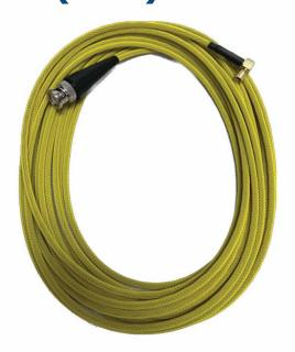
The BERG-122 is a 25-foot ultrasonic test cable designed for reliable signal transmission between flaw detectors and ultrasonic transducers. It features a BNC straight connector and a right-angle Microdot (MD) connector, providing an ideal solution for tight probe placements and mid-range inspection distances. The RG-174 coaxial cable offers flexibility and durability, while the flame yellow jacket ensures high visibility for safe use in both laboratory and field environments.
