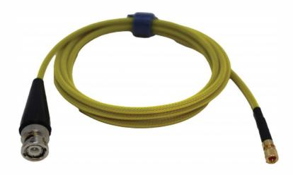
The BERG-120 is a 6-foot ultrasonic test cable featuring a BNC straight connector on one end and a Microdot (MD) straight connector on the other. It is designed for use in ultrasonic flaw detection, thickness gauging, and calibration. Built with RG-174 coaxial cable, the BERG-120 provides a lightweight, flexible solution for precise signal transmission. Its flame yellow jacket enhances safety and visibility in active inspection environments.
