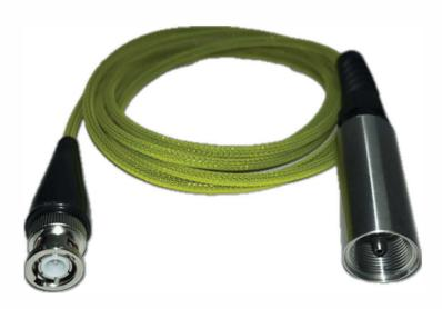
The BERG-116 is a rugged, waterproof ultrasonic cable designed for demanding inspection environments. Featuring a BNC straight connector on one end and a UHF straight connector on the other, this 6-foot cable delivers reliable signal integrity in both lab and field NDT applications. Its flame yellow jacket enhances visibility and safety, while sealed connector interfaces provide moisture protection during outdoor or high-humidity use.
