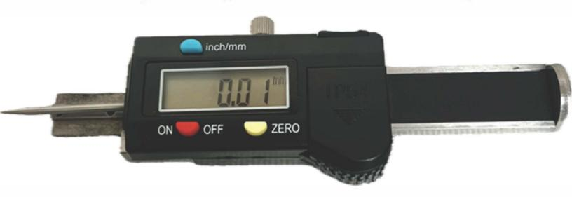
The BE-DPG-3 is a high-precision digital pit or depth gauge designed for measuring shallow pits, undercuts, dents or surface irregularities in metal, concrete or composite substrates. The instrument incorporates a hardened stainless-steel body, a spring-loaded finely-tipped probe, and a digital read-out, offering fast, reliable measurements in the field or workshop environment.
