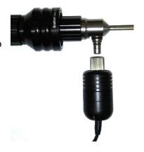
Plug the LXC-LED cable into the power jack on the bottom of the LXC.
