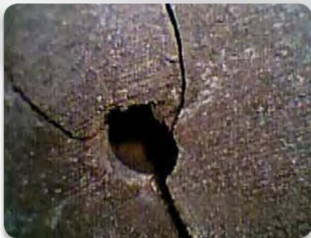
Using the optional Close-Focus Tip, fine cracks are detected inside a combustion chamber.
